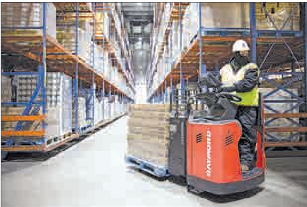
A new Raymond 8910 forklift powered by a lithium ion battery being used at a storage facility. (Submitted photo)
